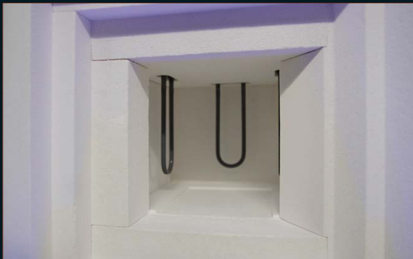
Combustion chamber of Zirkonofen 700 with \text{MoSi}_2 heating elements
